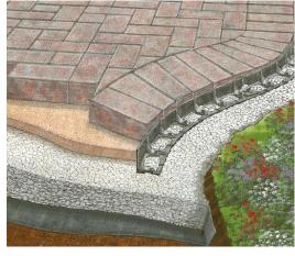
Different edge restraints: above, a plastic type sits on top of the compacted base, below a landscape timber defines the edge and holds bricks in place.
