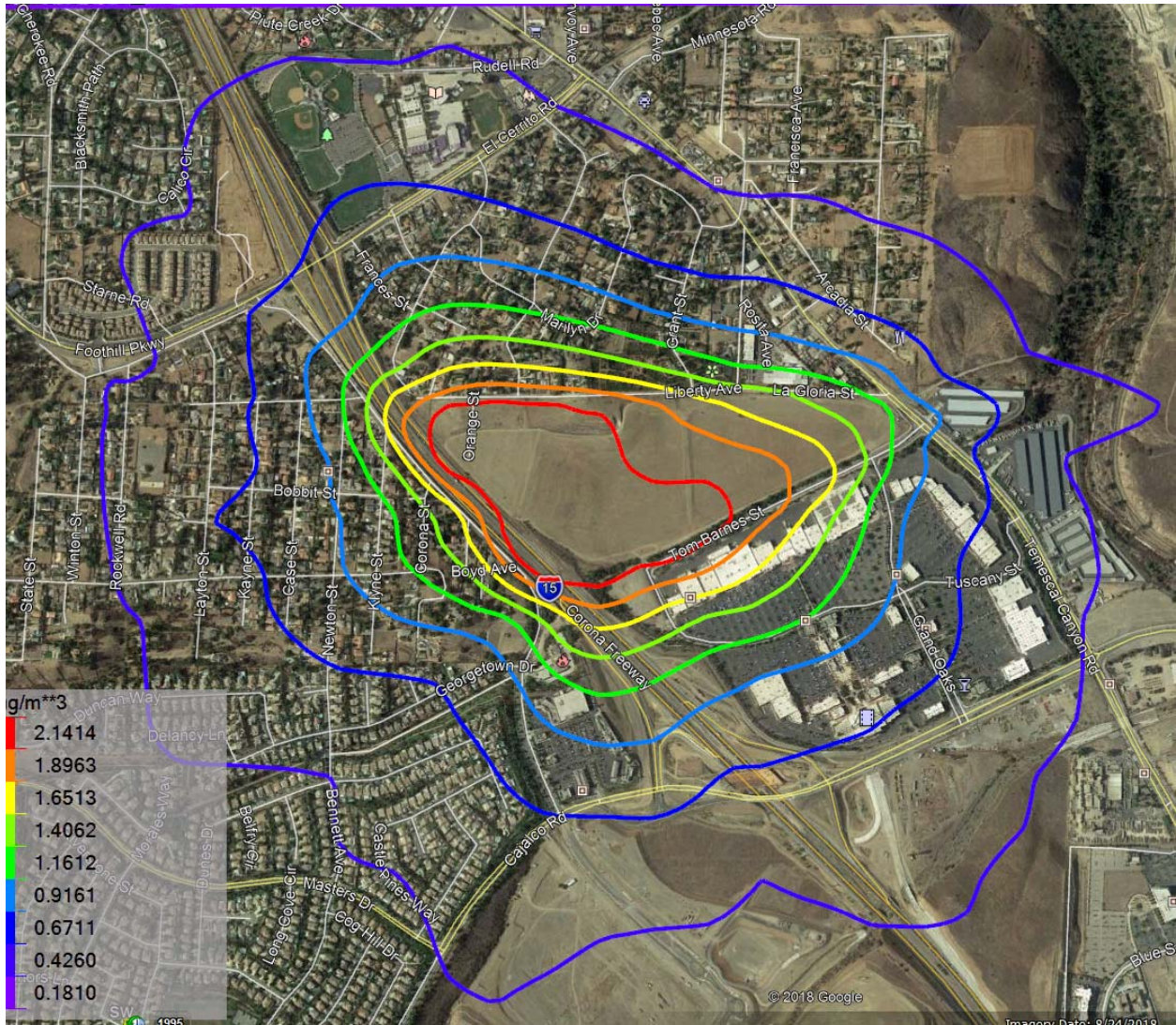
Figure 4-C: PM 10 – 24HR Maximum Construction AERMOD Plot
