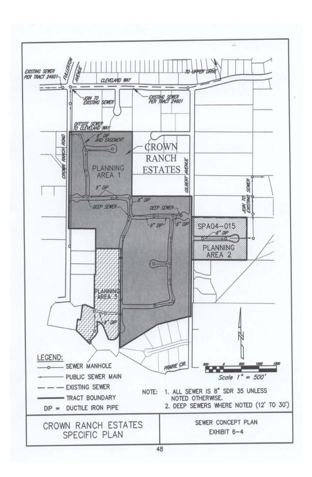
Due to topographical constraints on the site, it may be necessary to utilize deep sewers in portions of the site, ranging for 12 feet to 30 feet in depth, in order to properly sewer the entire site. All deep sewer lines shall be constructed of ductile iron pipe per City standards. The proposed Sewer Concept Plan is shown on Exhibit 6-4 and will be owned and operated by the City of Corona.
