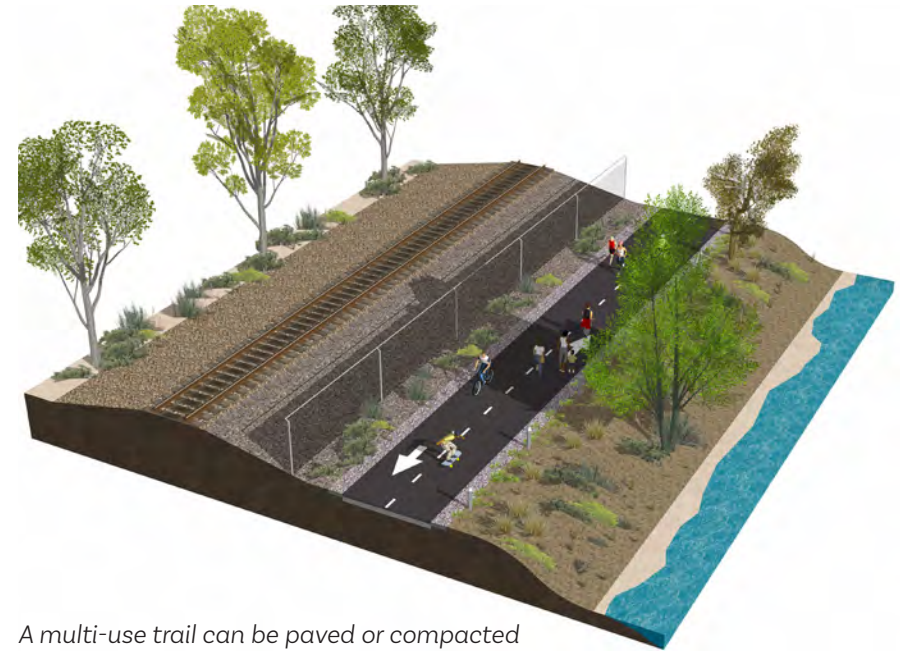
25-foot trail easement needed when next to a channel or a rail line
