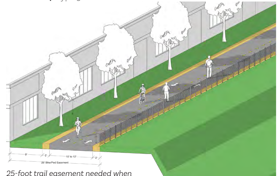
25-foot trail easement needed when next to a channel or a rail line
