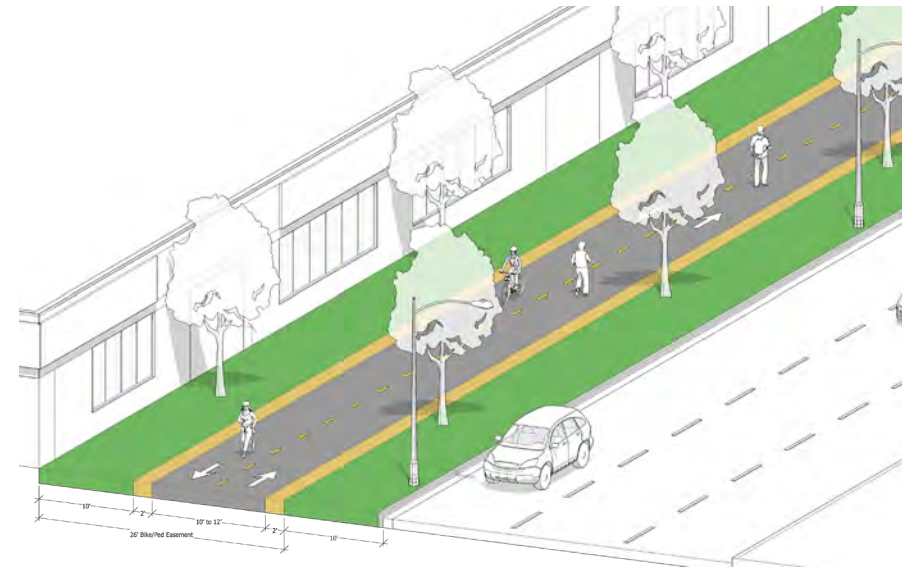
26' Trail Easement or portion of the Roadway Right-of-Way suggested
