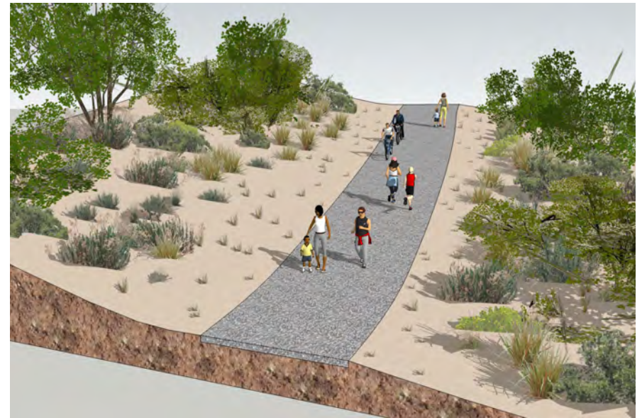
A Type 4 Trail can include a compacted 8-12' wide firm surface road that is not open to private vehicles but may be used by utility, maintenance, or emergency vehicles.
