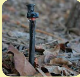
Bubblers - 85% efficient Work like a sprinkler but water does not spray out, it slowly bubbles out. Bubblers are generally placed at the base of individual plants.
