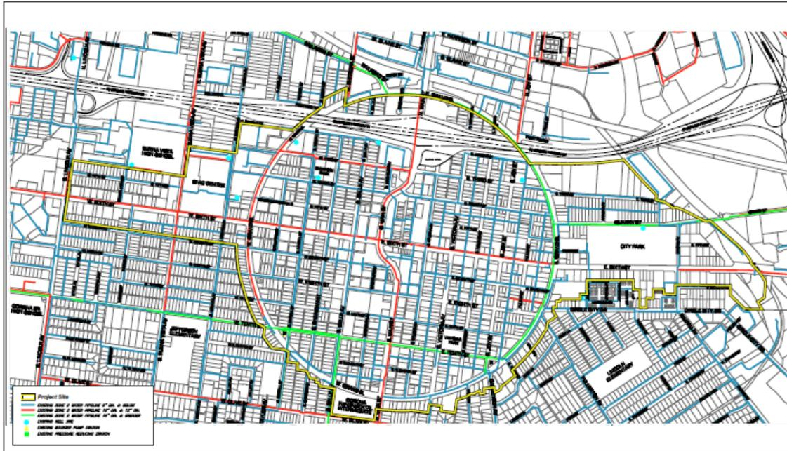
**Figure VI-A: Proposed Water System Improvements**
