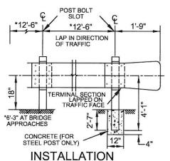
NOTE: GUARD RAILING FLARES AT BRIDGE APPROACHES SHALL HAVE A MINIMUM RADIUS OF 150'.
