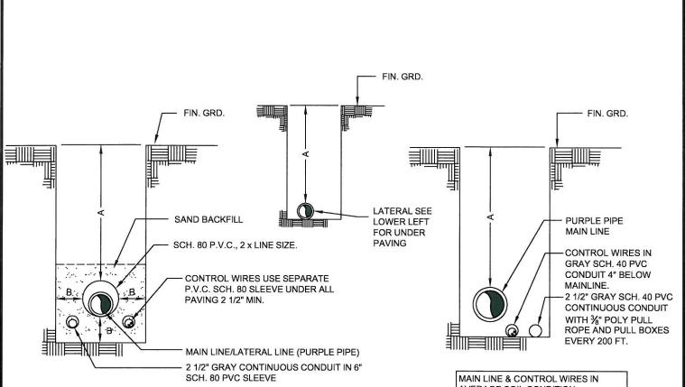
MAIN LINE & CONTROL WIRES UNDER PAVING
